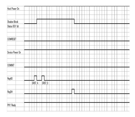
Figure 6.4 Response to a software reset
